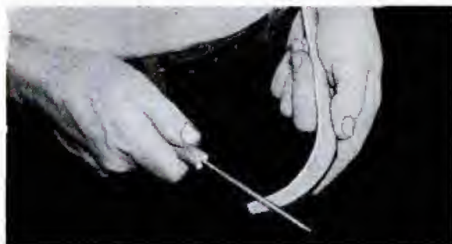
Upper photo, one of several types of plastic over-draw attachments. Center, cutting nocks (notches) in the recurve tips of a flight bow. Below, bowmakers finish the bow by dipping in tank containing varnish
